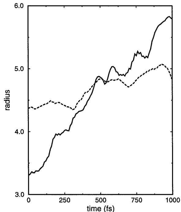
Figure 4. Gyration radius (Å) as a function of time for [HOHBr] - (H 2 O) 2 (solid lines) and [HOHBr] - (H 2 O) 6 (dashed lines).
